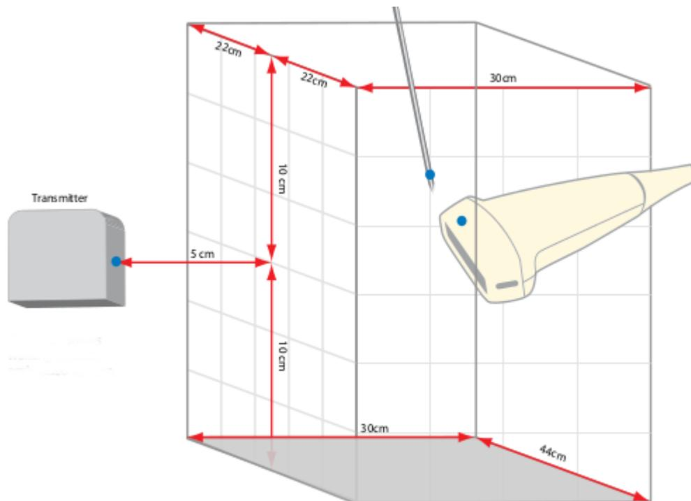
**Figure 1: Illustration of the SonixGPS system. Image courtesy of Ultrasonix.**
